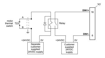
Figure 9 - Motor thermal switch circuit
